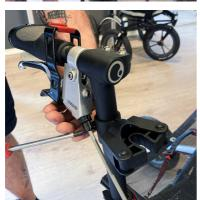
2 Snap the holder onto the upper part of the hand grip tube.
