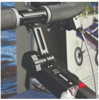
**B7.** Identify the circular front end of the light holder, with two slots for attaching the light.
