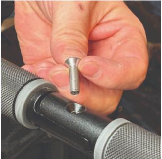
Al. Locate the screw at the center folding hinge of the U-shaped grip bar of the Veloped. Unscrew the screw with the included 4mm allen key and remove it.
